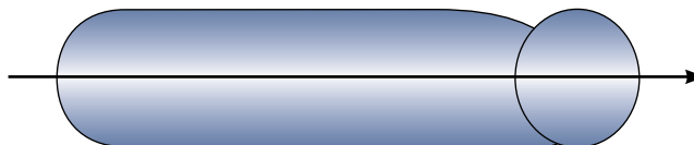
Path of a molecule through a leak path in laminar flow.
