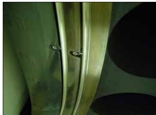
RPV O-FLEX™ Seals with installation clips
